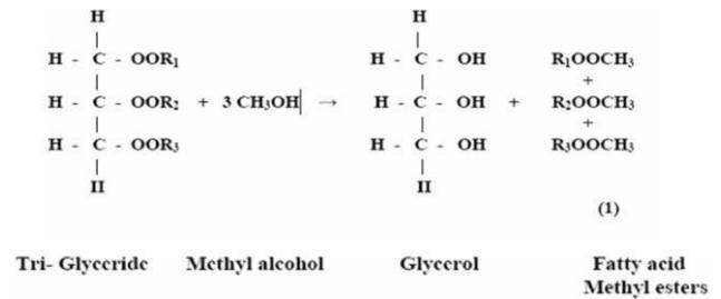
Figure 1 chemical reaction of the Tri-glyceride with Methyl alcohol
