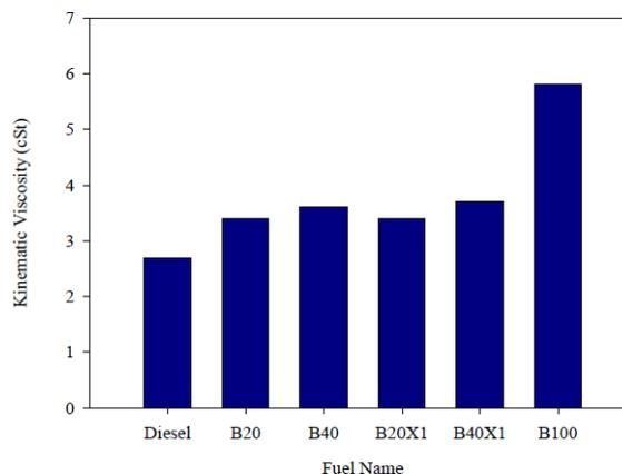
Figure 3 Kinematic Viscosity of Various Fuels Kinematic viscosity for pure Mahua bio-diesel and B20 are 5.8 cSt and 3.4 cSt respectively, whereas for diesel kinematic viscosity measured is 2.7 cSt. This is shown in figure 3 Mahua bio- diesel has 1.9 times higher kinematic viscosity compared to diesel. Density of Mahua bio-diesel is 0.824 g/cc where as diesel has density of 0.818 g/cc. Due to higher density of Mahua bio-diesel, specific fuel consumption will be less than diesel
