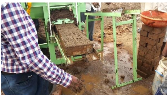
Fig 1 : Brick manufacturing process
