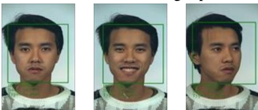
Fig. 1 Detection of individual "00690" faces from the Color FERET database with the Viola-Jones algorithm according to various poses and expressions visible on the face.
