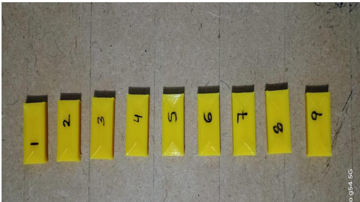
Figure 4: Hardness Specimen Prepared from 3D Printer
