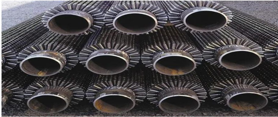
Fig. 3 Gilled Tube Type Economisers
