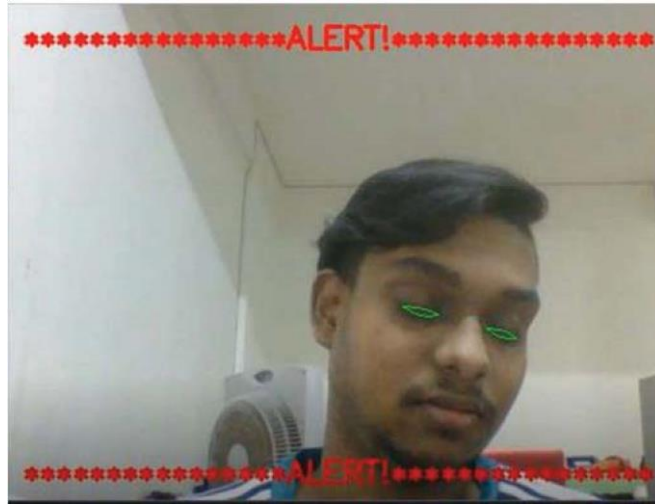
Fig. 10. Eye detection in microsleep condition.
