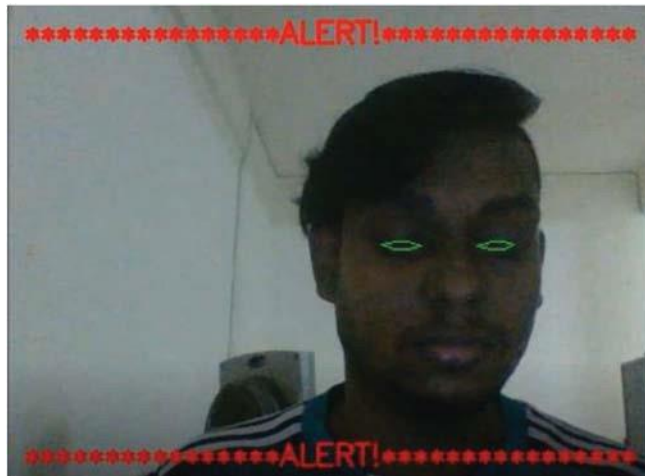
Fig. 9. Eye detection in dim light surrounding.
