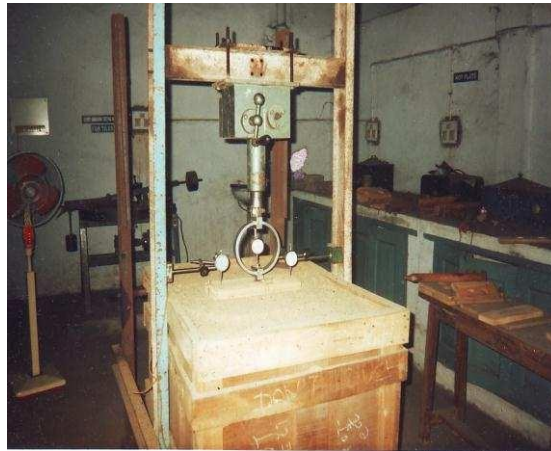
Fig. 1 Pile Load Test Setup
