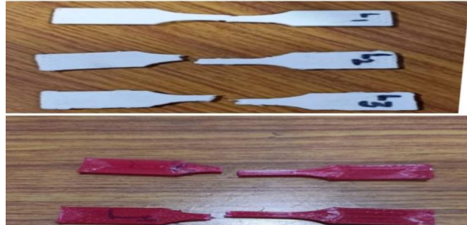
FIG-7, Specimens after Tensile Test
