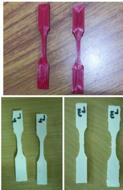
FIG -5, 3D PRINTED SPECIMENS V-TESTING
