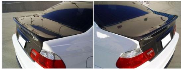
Fig. 1 – Carbon fiber trunk lid of BMW E46 M3 CSL.
